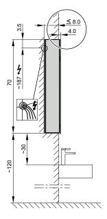
Unterputz-Montage Pose en encastrement Recessed mounting
