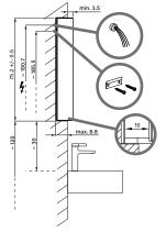
Pose en encastrement UP Recessed mounting
