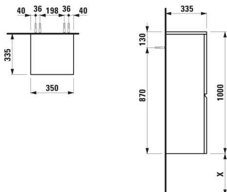
X = The exact height must be set during installation.
